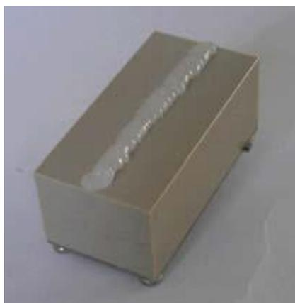
**Figure 10 Applying ultrasonic couplant**
